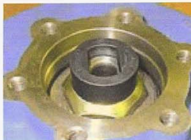
Figure 1 Pulley hub with coupler in place on shaft
