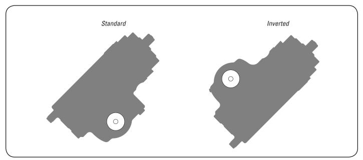
Gear Mounting Configurations
