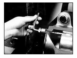
Turn adjusting screw assembly into housing
